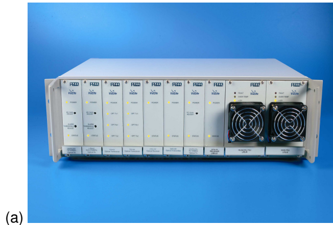
Figure 5 ViaLite Modules in (a) 19" 3U Rack Format, (b) 19" 1U Rack Format and (c) Standalone Format
