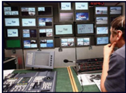
Broadcasters increasingly prefer to deploy temporary OB systems that incorporate a live fibre feed between remote receivers and the production suite. Wireless microphones are distributed throughout the auditorium or venue to capture live sound. At the remote receiver nodes, audio signals are converted into optical signals prior to transmission over single mode RF down-links to the production suite housed in the OB van.
