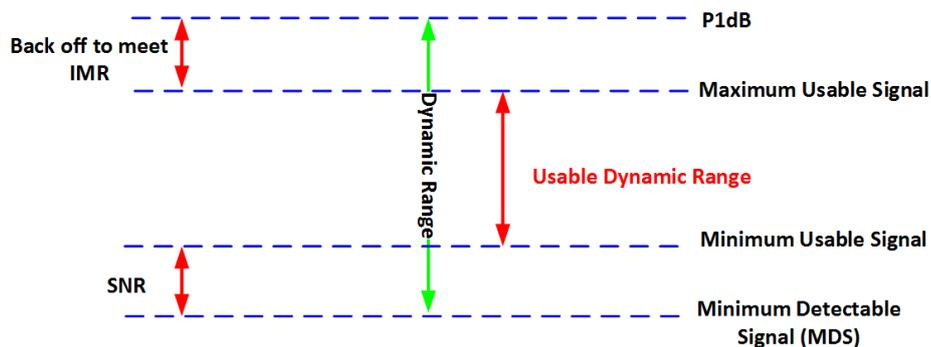
If you take a typical IMR of 40 dBc the maximum signal will be reduced by 8 dB, and at a typical SNR of 20 dB the minimum input signal is increased by 20dB, as shown below:
