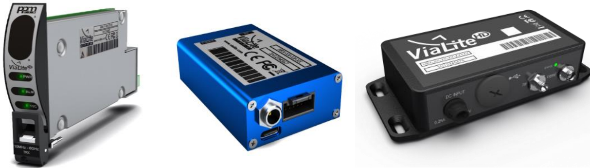
Figure 3. ViaLite Mil-Aero 6 GHz form factors: Rack Chassis Card, Blue OEM & Black OEM
