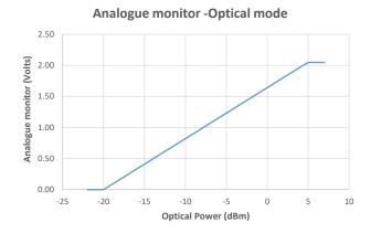
When configured to reflect optical power, 2V represents maximum rated optical power (typically 3.0mW). The analogue scale follows at -12.2dB per Volt.
