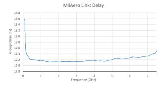
The delay through a short link (1m) is fairly consistent from 240MHz to 6GHz at 12.2ns. The extra delay seen in the link for low frequencies (<240MHz) is visible in the measurement data and is a feature of the optics and interface circuits that can't be avoided, though for any real-life fibre length, this difference becomes negligible at the equivalent of only 6m of fibre for the 40ns measured at 10MHz.
