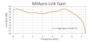
The link frequency response is fairly flat from 10MHz to 6GHz typically < +/- 1 dB. Usable gain is present up to 7GHz.
