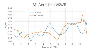
The VSWR of the transmitter input and receiver output is generally better than 1.4.
