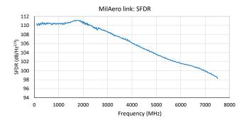
The SFDR of the link is a result of the noise figure and IP3 and is a good indicator of link dynamic range. This is important for links that transport wideband signals or signals with complex modulation types. The roll-off with frequency follows the noise figure response as stated earlier.
