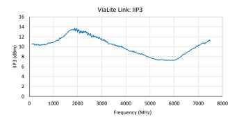
The input IP3 of the link is fairly consistent with frequency and is directly influenced by the transmitter gain setting which can be traded with noise figure to suit the application. The measurement here is from a link incorporating the low gain transmitter. This parameter does not change with link loss though it does change with link length if presented with chromatic dispersion. Please consult your sales representative for long distance designs that mitigate for dispersion effects.
