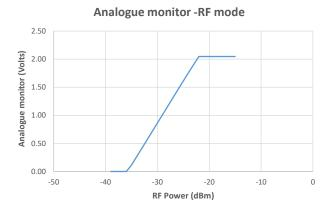
When configured to reflect RF power, 1.5V represents 10dB above the measurement noise floor. The RF detector system is for indication only as the dynamic range is fairly limited. The example given here is for a standard gain transmitter module.
