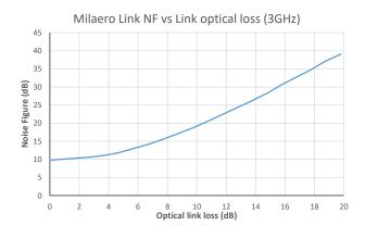
The Noise figure degrades with increasing link loss. In the high gain link measurement shown adjacent, the noise figure increases slowly for the first 4-5 dB of optical loss and then increases 2:1 with optical loss. Minimising link loss is crucial to maintain best performance.
