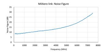
The Noise figure can be traded with linearity using the transmitter gain settings to best suit the application. The measurement here is from a link incorporating the high gain transmitter. The noise figure of the link increases with frequency as a result of the laser technology so must be considered when selecting the gain.
