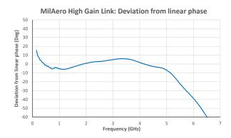
The deviation from linear phase is within +/- 7 degrees from 350MHz to 5GHz. At the frequency extremes, the phase deviates as shown in the chart.
