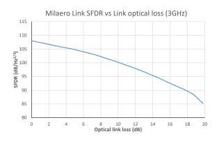
The SFDR degrades with link loss as a result of the increasing noise figure. Further degradation with link length can be expected if presented with chromatic dispersion. Please consult your sales representative for long distance designs that mitigate for dispersion effects.
