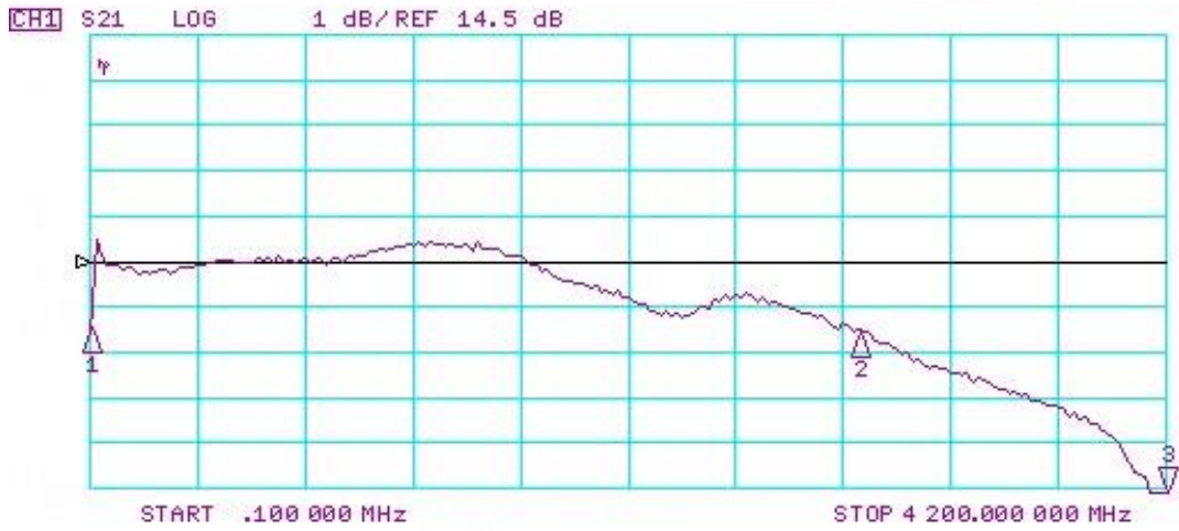
Gain versus frequency, gain set to minimum, gain 14.5dB
