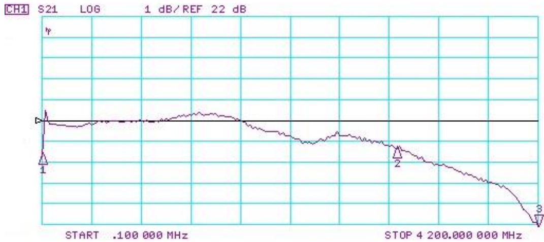
Gain versus frequency, gain set to median, gain 22dB
