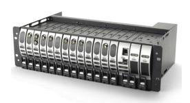
The HWDR cards are available with *ViaLiteHD* blind mate, which allows all cables to be connected at the rear of the chassis when installed. Blind mate also allows configuration changes to be completed without disturbing the connections and very fast changeover of cards; enabling five 9s reliability.
