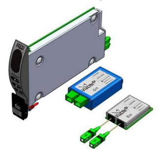
ViaLiteHD fiber optic links are available in three hardware formats: rack mounted cards, m-link modules and Edge OEM modules. A fully populated 19" 3U ViaLiteHD rack supports up to 26 links and accepts 13 RF and accessory cards plus an M&C card and dual power supply modules. A 1U chassis accepts three RF cards or two RF cards plus an M&C card.
