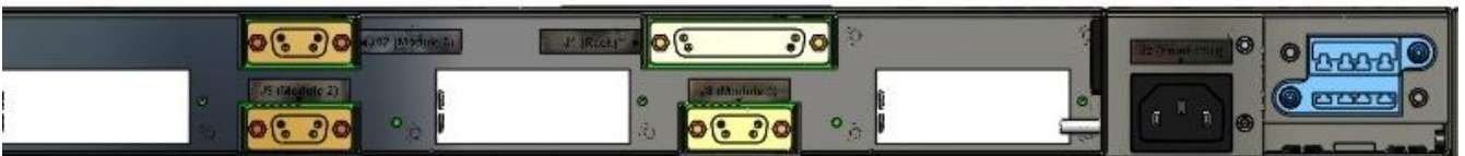
HRK1S View of interface connectors on the rear of the chassis (no modules fitted)
