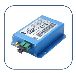
Many Network Time Protocol (NTP) server networks are required to maintain extremely accurate clock systems for timing synchronization. The *ViaLiteHD* GPS link is ideal for providing a remote GPS signal or derived timing reference to equipment positioned where no GPS signal is available. For example inside a building, tunnel or underground mine. By using fiber instead of traditional coax cable, longer distances are possible with no RF loss and zero introduction of noise.
