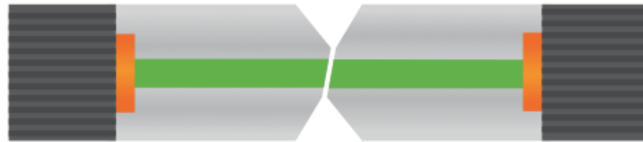
Angled physical contact connector
