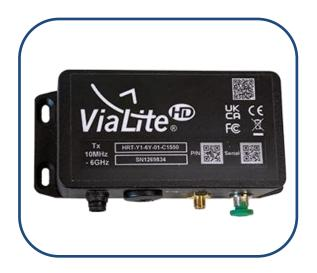
The Black OEM Module is an outdoor rated RF over fiber link which covers a wide frequency range from 10 MHz to 6 GHz. With this range in frequency, the OEM unit can be used in a wide variety of applications, such as Broadcast, Satcom, GPS/Timing and Mil-Aero. With an IP66 rating, the module is suitable for installations in harsh environmental conditions, without requiring an outdoor enclosure.
