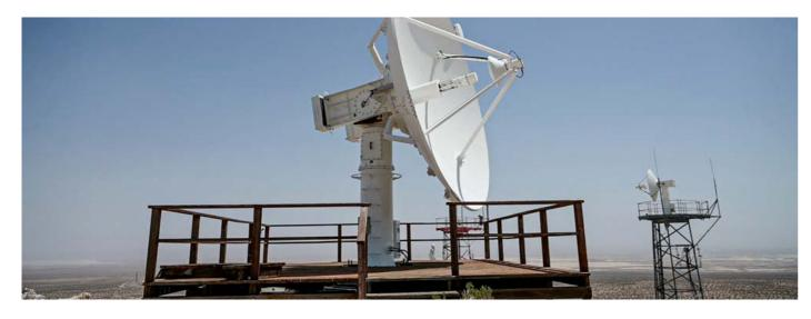
Using RFoF, these antennas can pass the telemetry data back to a central control building where it can be losslessly split to multiple analysis and monitoring workstations for processing, whilst control workstations can pass control signals back to the antenna positioners to ensure alignment with the platform under test.
