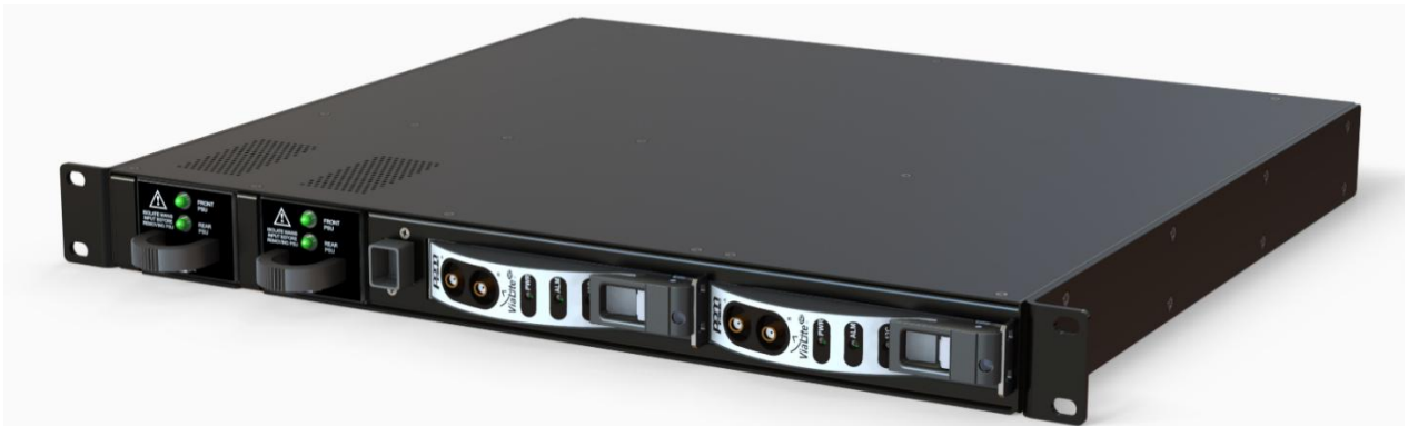
GPS Splitter Rack accommodates up to two single or dual GPS RX modules, one embedded control module and two front mount power supplies
